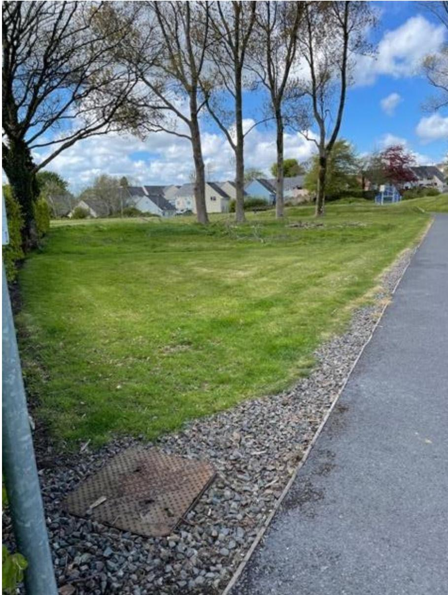
This is the opposite view looking from the upper manhole towards the ground of trees. The existing drainage which has failed runs through the centre of these trees. The proposed new route is between these group of trees and the single tree seen on the left of this photograph.
